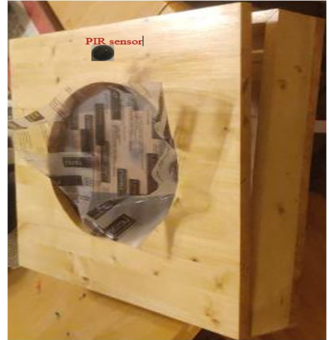
Smart window with PIR sensor placed outside
